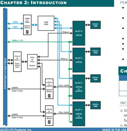
PCIe/104 is part of the PC/104 family of standards, and incorporates PCI Express, USB, SMBus and other data channels in the stack, not a single bus (ISA or PCI) as in previous standards. It is intended to be used in environments where a truly rugged computer system is required. PCIe/104 allows consumers to stack together boards from a variety of COTS manufacturers to produce a customized system ruggedized against the stresses of embedded environments.
