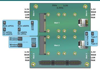
The 104e-mPCIe-4A modules need the following configurations:
